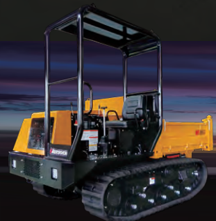
MST-300VD Max. Payload 2,500kg Tier4 Interim / EU Stage IIIA
