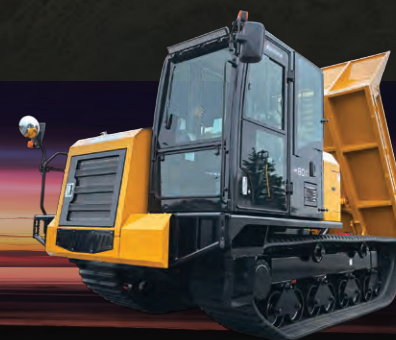
MST80C Max. Payload 8,000kg Tier4 / EU Stage V
