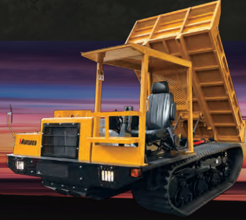
MST-800VD Max. Payload 4,800kg Tier2 / EU Stage II
