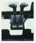
Electric control travel levers enable smooth and stress-free operation for operators. Furthermore, by expanding the available floor space, it also enhances overall livability.
